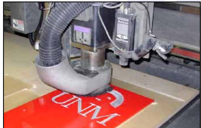
The MultiCam Router features MultiVision digital registration for quick and accurate alignment.
